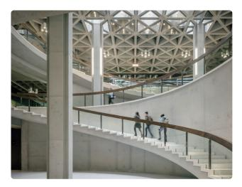
On the ground floor, large openings have been formed in the original marble-clad walls of the entrance hall. A generous passageway leads to a large circular hall that has been cut through the floors of the podium at the centre of the plan. These alterations bring light into the building, connect the various levels of the building and provide new shared spaces for the users.
