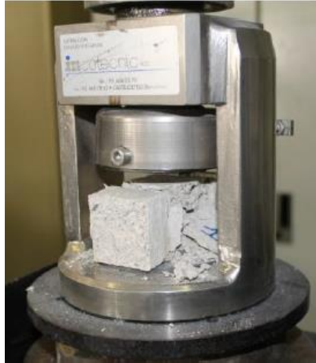
Figure 23: Mortar compression cube test failure (Canella, 2014).
