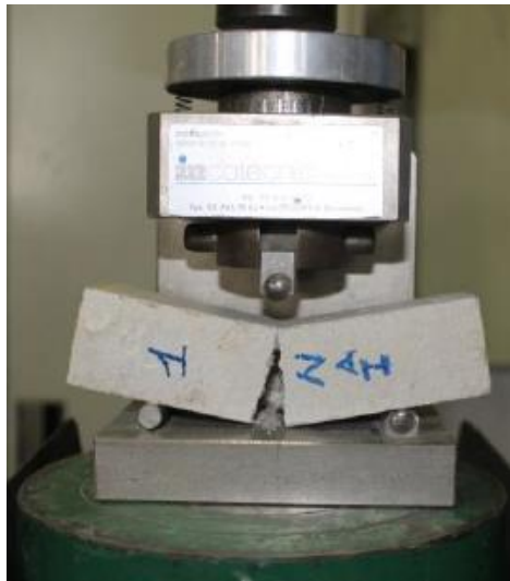
Figure 30: Mortar three points bending test failure (Canella, 2014).
