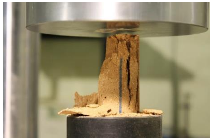
Figure 35: Brick compression cylinder test failure (Canella, 2014).
