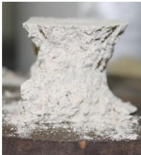
Figure 49: Typical Hourglass failure mode presented on brittle materials subjected to uniaxial compression (Canella, 2014).
