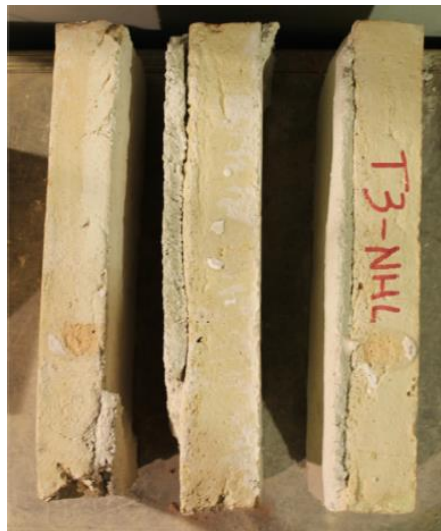
Figure 59: Experimental failure for triplets shear tests: internal crack formation (Marastoni, 2016).
