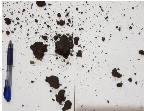
Figure 5. 6. Soil qualitative tests part 2; (a) ball pressing test: five ball samples and finger pressure applied after drying, and (b) ball dropping test: balls broke into several relatively big pieces indicating an adequate amount of clay for earthen construction
