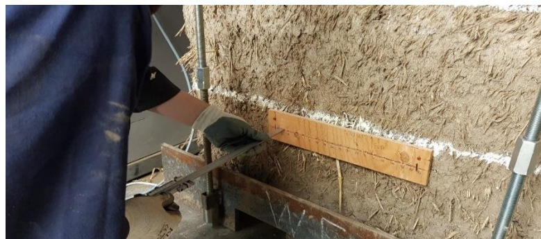
Figure 5. 53. Measurement of the cut depth.
