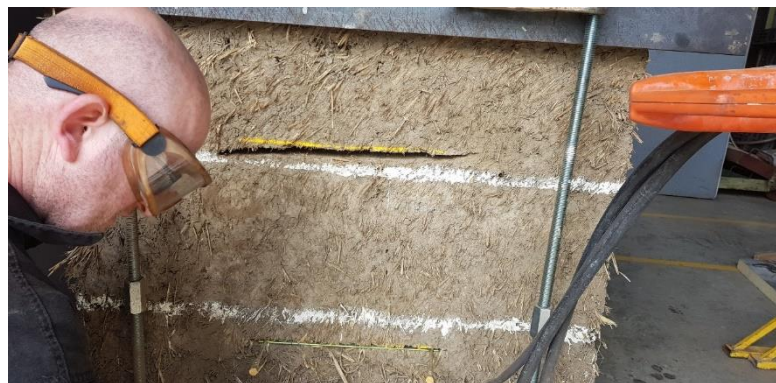
Figure 5. 61. Second cut done in the first walette.
