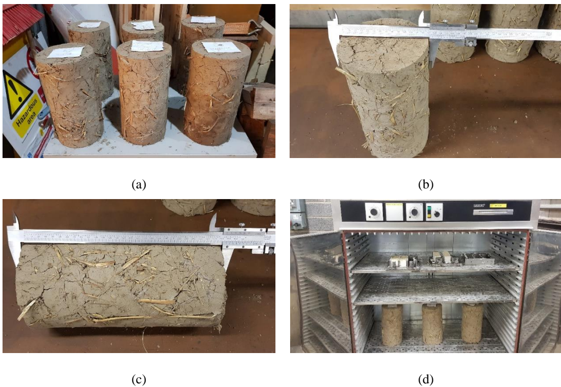
Figure 5. 30. (a) Cylinders' storage in the laboratory, (b) measurement of cylinders' diameter, (c) measurements of cylinders length and (d) oven drying of cylinders.
