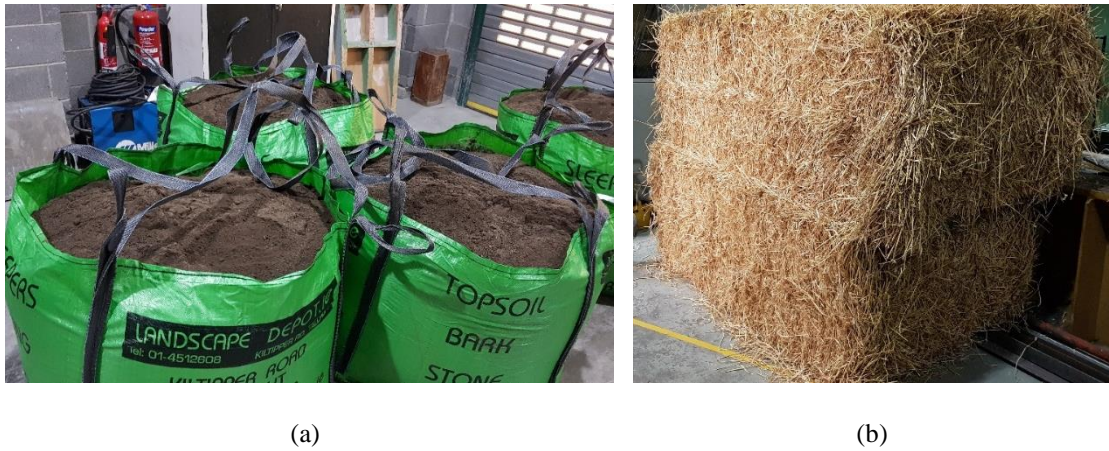
Figure 5. 3. Soil (a) and wheat straw (b) locally sourced for the construction of the cob wallettes.
