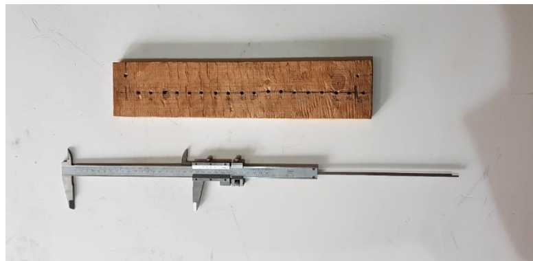
Figure 5. 47. Timber template and calliper Vernier used to measure the depth of the cut.
