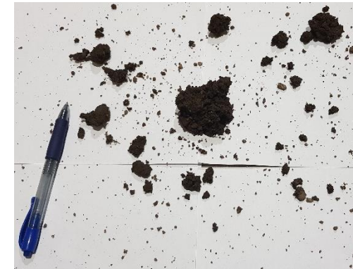
Figure 5. 6. Soil qualitative tests part 2; (a) ball pressing test: five ball samples and finger pressure applied after drying, and (b) ball dropping test: balls broke into several relatively big pieces indicating an adequate amount of clay for earthen construction
