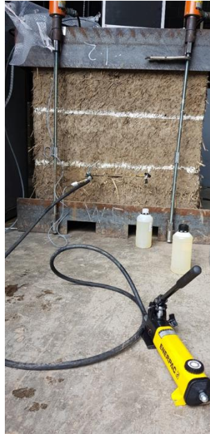
Figure 5. 55. System purged and ready to start applying pressure increments.
