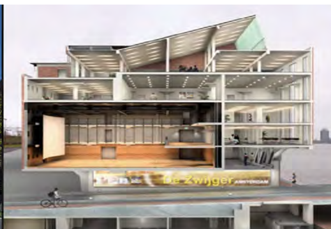
The missing floors were incorporated in the main room
